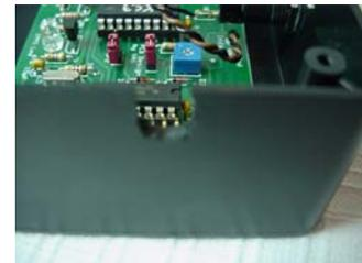
Slide the Serial cable down into the slot in the enclosure making sure that the flat portion of the strain relief is facing upward and is oriented horizontal with the top of the enclosure.
