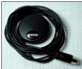
A GPS unit and a phono cord complete the system. The GPS can also be used to find the observing location.
